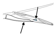
3. Grip tightly and press on the arm/blade joint from beneath and separate the blade from the arm.
